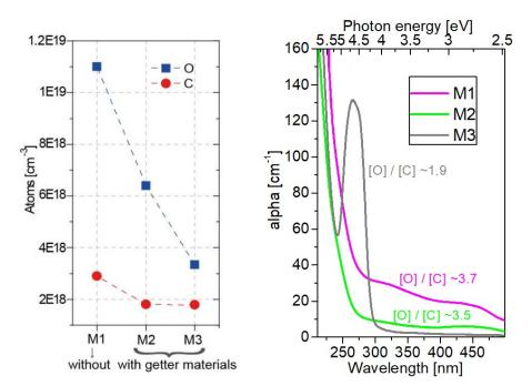
Fig. 3: Carbon and oxygen concentrations in AlN bulk crystals grown without and with getter materials (left) and corresponding optical absorption spectra in the UV range (right)
