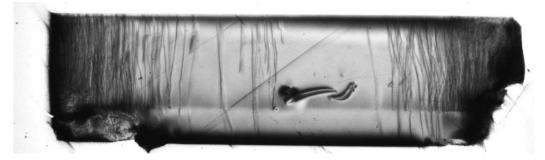
Fig. 1: 11-20 transmission X-ray topograph of an AlN wafer a-plane cross-section (the lower part is the seed; the width of the cross-section is about 10 mm)
